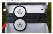
For micro cable size 3.0 - 4.5 mm NanoFlow MAX adaptor plates and MAX steel wheel applies.
